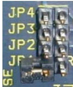
To select GEN Mode, take the jumper OFF and place it over only one pin.
