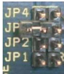
To select SHALLOW Depth-of-Discharge, leave the jumper OFF and placed over only one pin.
