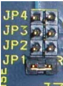
To select UPS MODE, leave the jumper ON (This is the default configuration.)
