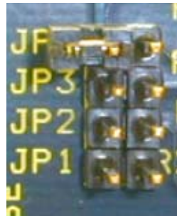
Jumper OFF: Do not remove the jumper unless instructed to do so by an authorized Xantrex Customer Service Representative.
